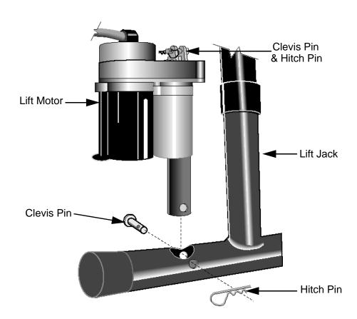
6. Remove the clevis pin, then pull the lift jack out of the column. Set aside the defective lift motor. Return the treadmill to an upright position.
