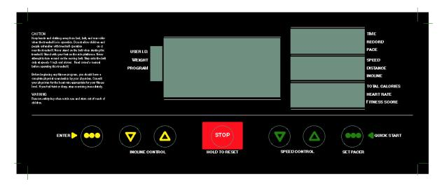
7. Remove the safety key from the upper display module while you watch the right display window. Return the safety key to the upper display module. If SAFE OFF is displayed when the safety key is removed and SAFE ON is displayed when the safety key is replaced...
